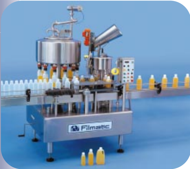
Filmatic's new generation flexible level filler; uncomplicated entry-level technology.
